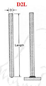
When ordering, specify Type, Diameter, Before Weld Length, Material, Quantity, and Part Number Example: D2L 1/2 x 18-1/8": Mild Steel: 5000 pieces: #101064765
